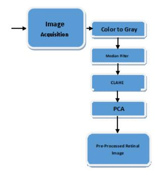
Figure 7. Block Diagram of the Proposed Pre-Processing Technique.
